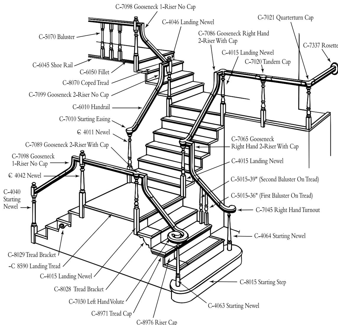
**BALUSTER** - A vertical member, used to fill the open area between the railing and the floor or tread, adding safety, support and stability to the balustrade.
